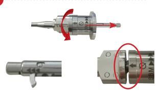
Pull the plunger and turn the graduated knob between 9 and 9.5 to remove the blade and leave a gap between the knob and the plunger.
