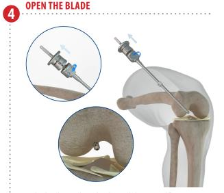
Turn the knob to select the desired diameter (from 6 to 11 mm, every 0.5 mm) and extend the drill blade.
